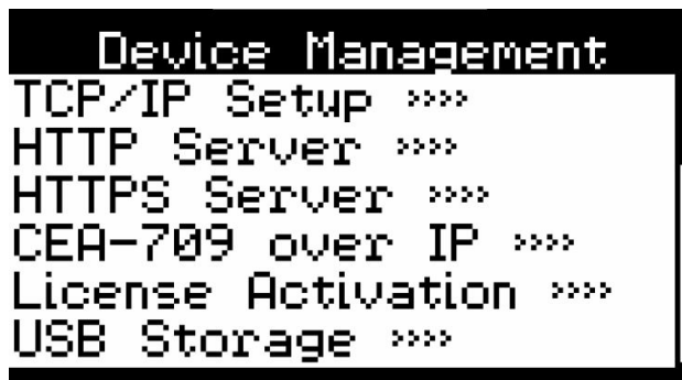
Figure 21. Device management menu on the LCD user interface.
